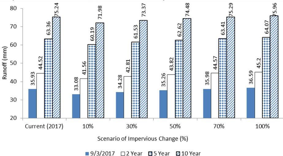
**Figure 9.** The results of estimated runoff levels at Building D pond sub-catchment responding to different scenarios for [1] the percentage of impervious areas, and [2] rainfall intensity.
