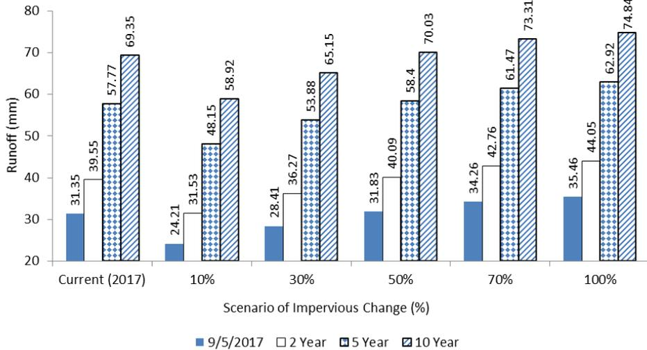
**Figure 10.** The result of estimated surface runoff volume level at the STEM building sub-catchment responding to different scenarios for [1] the percentage of impervious areas, and [2] rainfall intensity.
