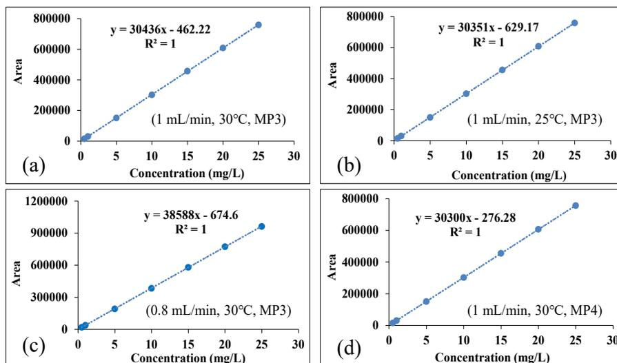
Figure 8: Calibration curve of standard caffeine observed by HPLC Arc™ Water parameters: (a) initial, (b) change column temperature, (c) change flow rate, and (d) change mobile phase.
