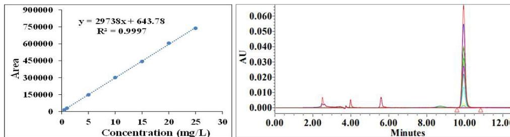
Figure 5: Calibration curve of standard caffeine at concentrations between 0.5 to 25.0 mg/L (n = 7) and overlay chromatogram with Sample 01
