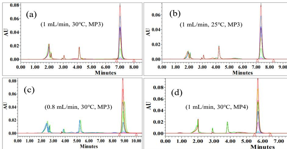
Figure 7: Overlay chromatogram of standard caffeine and Sample 01 after minor change on HPLC Arc™ Water parameters: (a) initial, (b) change column temperature, (c) change flow rate, and (d) change mobile phase.
