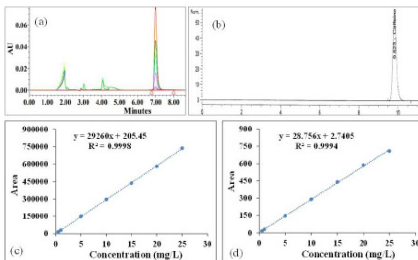
**Figure 4:** Chromatogram and a calibration curve of caffeine observed by (a)&(c) HPLC Arc™ Water equipped with ZORBAX C18 column and (b)&(d) HPLC Agilent 1100 equipped with InertSustain C18 column
