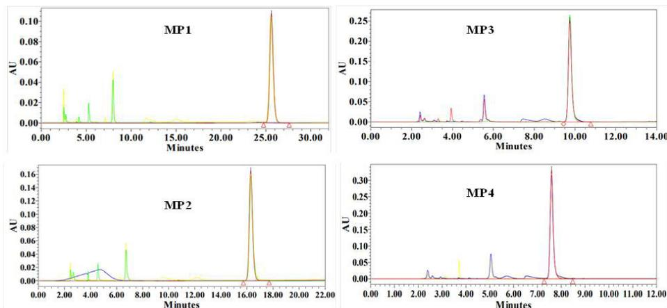
Figure 1: Overlay chromatogram of blank, standard caffeine, Sample 01, and Sample 07 respected to mobile phase composition
