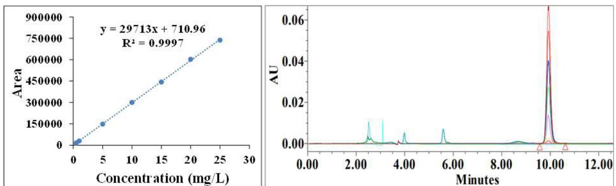
Figure 3: Calibration curve of standard caffeine at concentrations between 0.5 to 25.0 mg/L (n = 7) and overlay chromatogram with Sample 01
