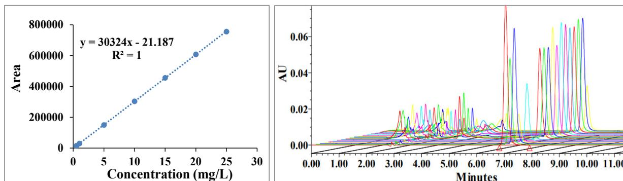
**Figure 9:** Calibration curve of standard caffeine at concentrations between 0.5 mg/L to 25.0 mg/L (n = 7). HPLC Arc™ Water and ZORBAX C18 column (flow rate 1.0 mL/min, 30°C, mobile phase MP3).
