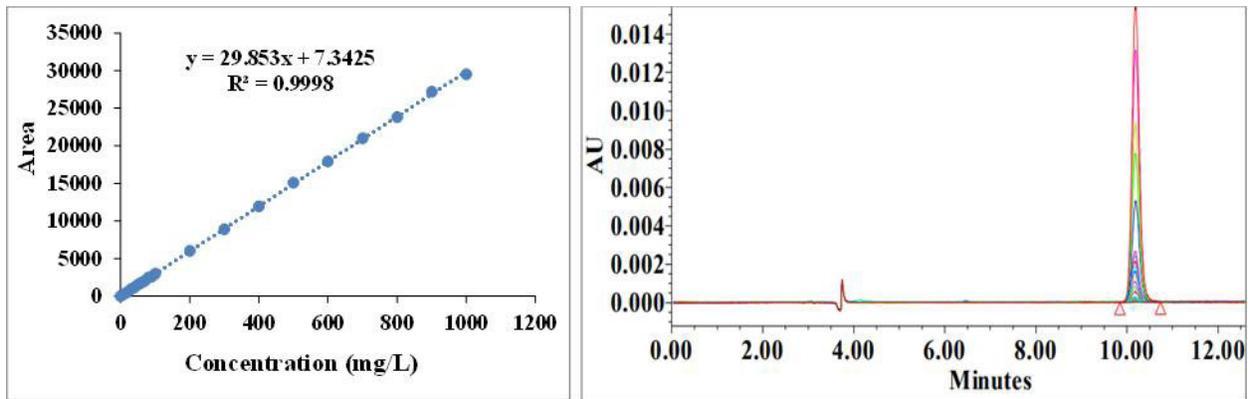
Figure 2: Calibration curve of standard caffeine at concentrations between 10 µg/L to 1000 µg/L (n = 19) and their overlay chromatogram
